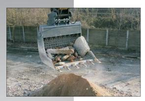
The "DASIE" screening bucket can be used as a hoe dipper for excavation or loading, simultaneously screening the material in the screening bucket. It screens all material on the construction site without plugging, effortlessly and effectively.
