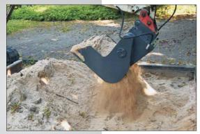
The "DASIE" screening bucket is used in landscaping for excavating paved roads with the simultaneous recovery of cobblestones, or for cleaning and aerating play sand and topsoil.
