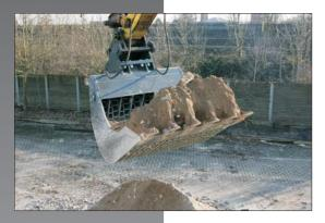
With the "DASIE" screening bucket, you can effectively separate and reuse all construction site materials such as building rubble, mixed construction waste, soil, slag or incineration residue. You gain storage volume while saving on transportation and landfill costs.
