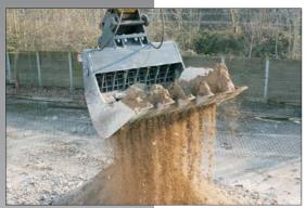
The "DASIE" screening bucket is ideal for landscaping, road building and sewer construction, demolition and quarry applications. Screening building rubble, soil and, in particular, the economical recovery of usable stone material suitable for processing significantly improves your bottom line.
